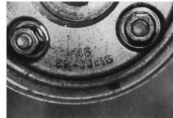
FIGURE 20-28 The size of the wheel is usually cast or stamped into the wheel. This wheel is 5 1/2 in. wide. The letters JJ refer to the contours of the seat area of the wheel.
